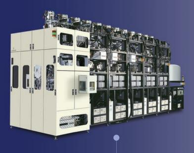
The 200 Lean magnetic media deposition system is used by disk media manufacturers worldwide and has an installed base of over 110 systems.
